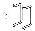
SWB, mounting brackets When not using the filter section the main unit is suspended from the wall or ceiling using brackets SWB (fig 2). Brackets are extra and supplied as a pair.
