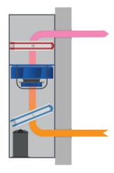
CDP 40T, 50T and 70T are designed for installation in an adjacent room and are supplied with a through-the-wall duct kit with supply and return air grills (accessory).
