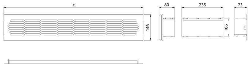
The duct kit includes an extension for wall thickness from 70 to 366 mm.
