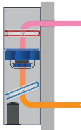
CDP 40T, 50T and 70T are designed for installation in an adjacent room and are supplied with a through-the-wall duct kit with supply and return air grills (accessory).
